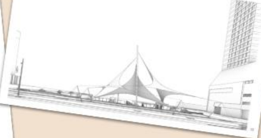
Tensile Shader - Columns are used to elevate the sails from the ground making the structure more compact
