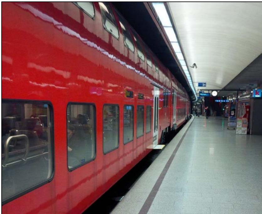
Figure 58: The Zurich S-Bahn bi-level cars, as shown, make use of doors on the lowest levels, allowing level boarding to meet accessibility needs
