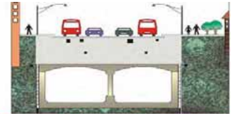
Step 4: Removal of Decking - Street Restoration When the finished construction is close to the surface, the temporary decking is removed and all surface amenities (e.g. roads) are reinstated.
