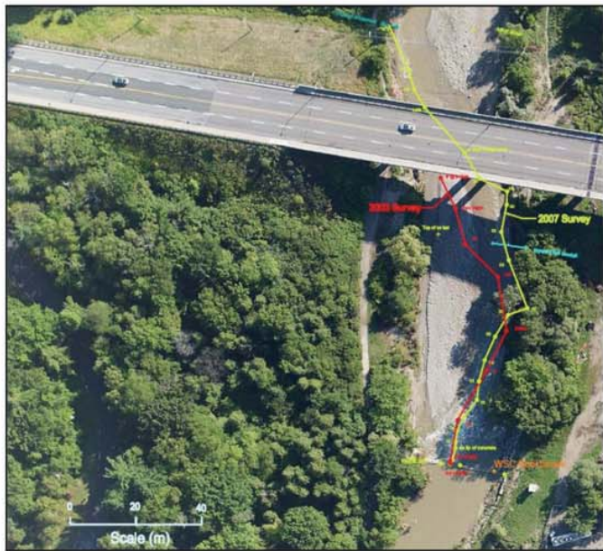
Figure 4. 2003 and 2007 survey showing the change in thalweg location near Morningside Avenue.
