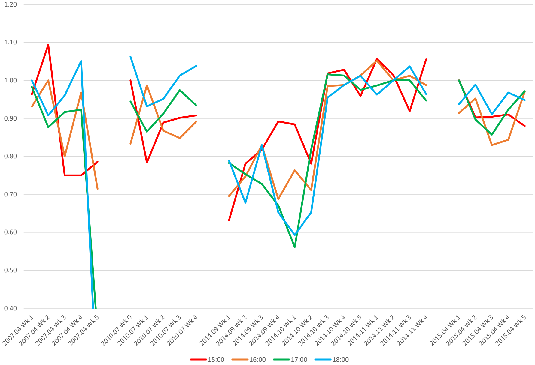
512 St. Clair Ratio of Vehicle Counts EB at Dufferin vs Keele Weekday Afternoons
