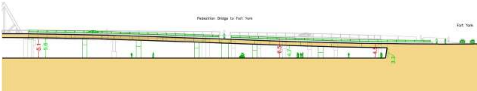
West elevation of the new bridge superimposed on the existing (from the ESR, enhanced by DTAH)
