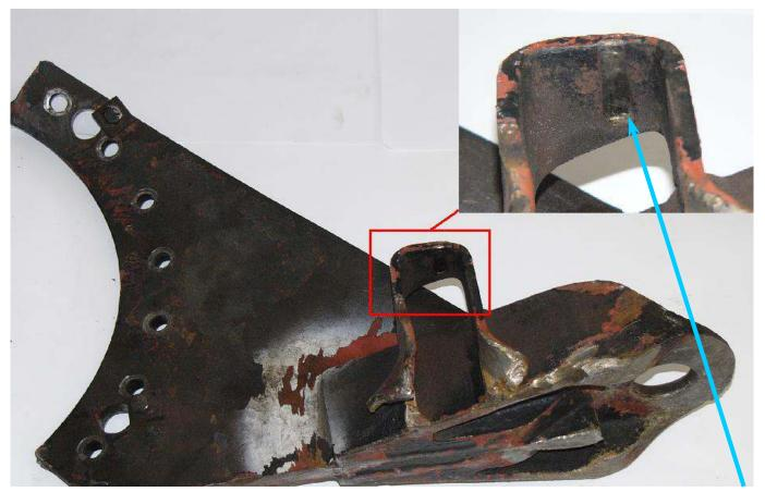
Contact mark inside "U" bracket significant evidence of vertical impact of torque arm on safety pin.
